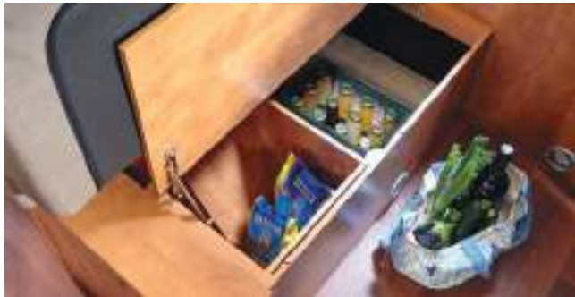
▲ There is a large storage compartment beneath the living area seat bench. It is easily accessible using a patented fitting, and can be opened without removing the seat upholstery.
