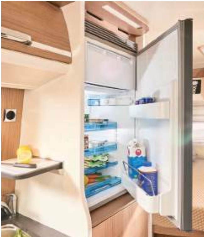
▲ The absorber fridge, which has been exclusively developed for Malibu, can be operated with gas, 12 V or 230 V.
