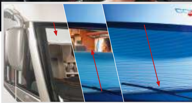
▲ Multi-functional insulating pleated windscreen blind, can be operated horizontally to allow it to simultaneously act as a sun blind, for privacy protection and as a blackout blind with insulation. From the chic e-line onwards, pleated windscreen blind with programmed privacy and sun visor function as standard.
