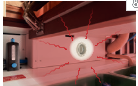
Truma Combi 6 heat storage heating system with numerous warm air outlets in the entire double floor, the living area, the rear garage, the driver's cabin and the cold-sensitive door entrances
