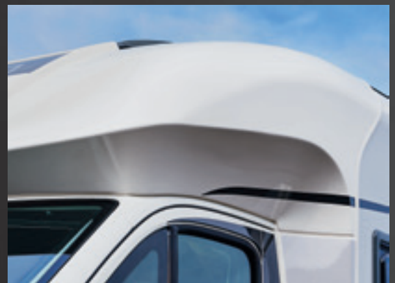
Carthago front shroud combines elegant design and high quality GRP construction. Thanks to the two shell insulation, the Carthago semi-integrated motorhomes guarantee the best living climate, even at low temperatures.
