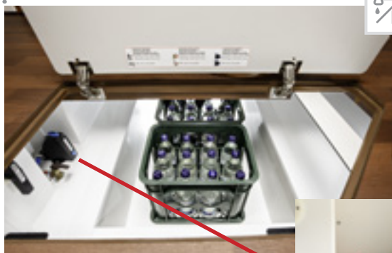
Central water drain in the double floor – can also be operated from the outside through the main cabin door
