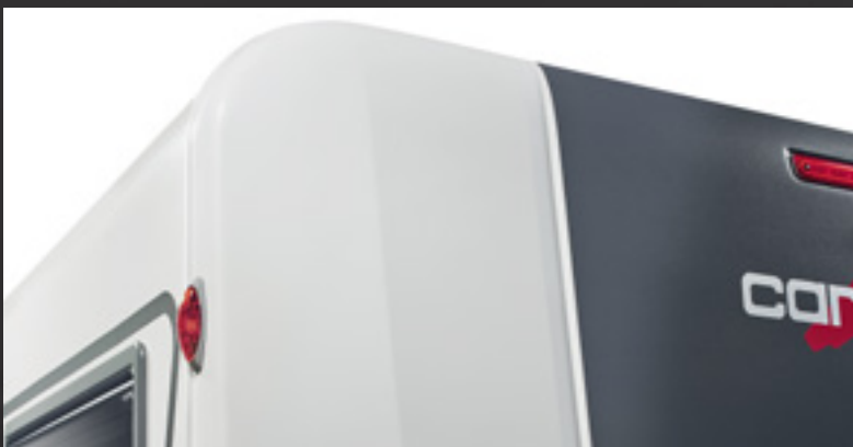
The Carthago curved roof Carthago awakens emotions with its unique and elegant design and the curved roof which is typical of the brand. It also increases the torsion resistance of the body, and there is less susceptibility to side wind. The perfect combination of design and practicality!
