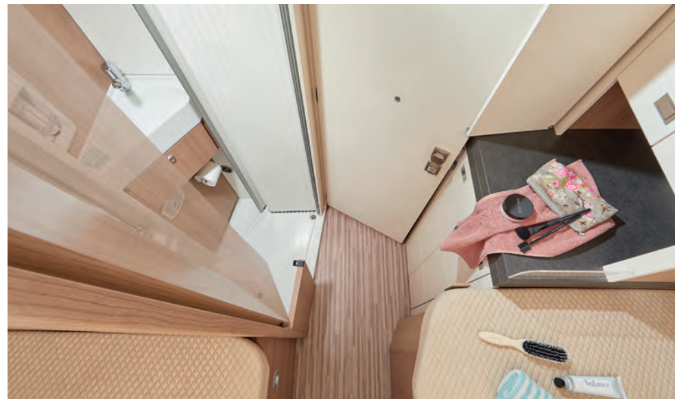
▲ Even more freedom of movement is created by means of the washroom wall, which swivels into the washroom.
