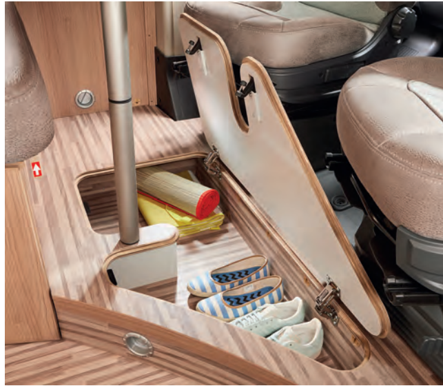
▲ Large storage compartment in double floor of lounge seating area with hatch and high quality hinges – quick and easy to access thanks to “One touch access”.
