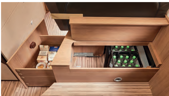
▲ Additional kitchen storage space is provided by the large storage drawer opposite the kitchen and the large storage compartment beneath the living area seat bench, which is accessible from above without having to remove the upholstery.
