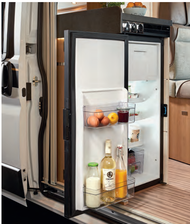
▲ The powerful 84 l compressor fridge is integrated at the front of the kitchen in the entrance area. It is therefore conveniently accessible from both inside and outside.
