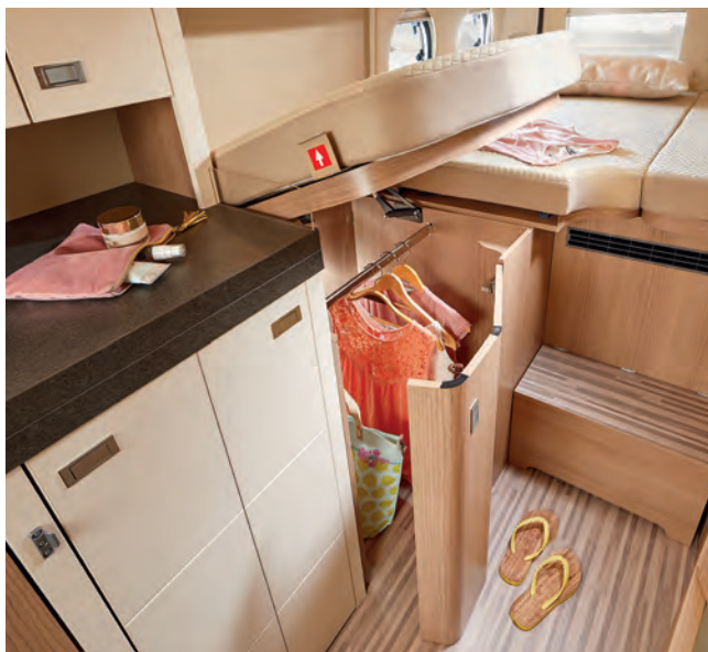
▲ Extra-large wardrobe beneath the lengthways single bed at the driver's side, conveniently accessible from above and the front.
