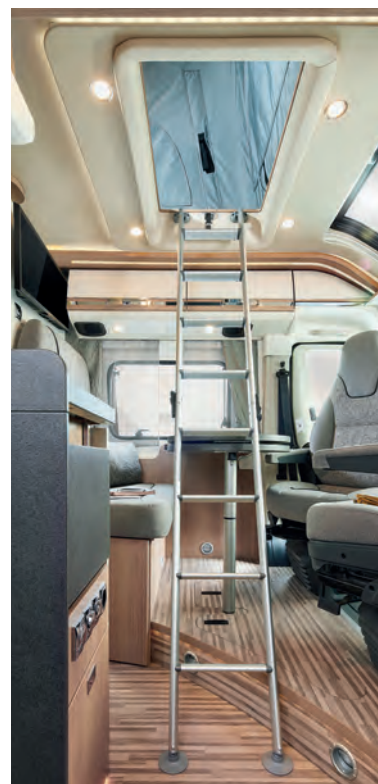
▲ Thanks to the access ladder, roof access is easy. If the ladder is not in use, it can easily be taken apart for stowing away.
