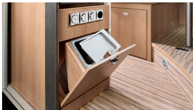
▲ The waste bin is separately integrated in the kitchen units, and is accessible from the outside and also from the living area.
