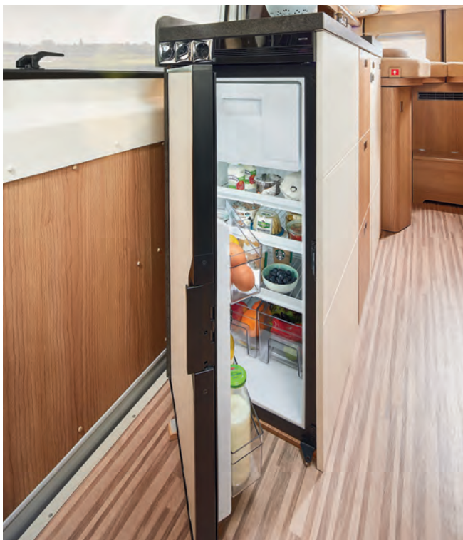
▲ The powerful 84 l compressor fridge is integrated at the front of the kitchen in the entrance area. It is therefore conveniently accessible from both inside and outside.
