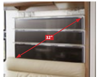
TV pull-out system for 32" LED flat screen behind side sofa backrest
