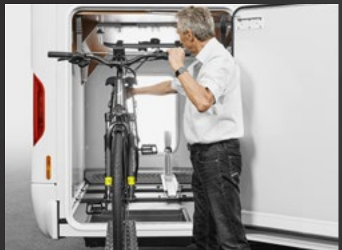
Loading height extension by simply swinging up the interior rear bed with one hand and the additional sunken floor recess (making a handlebar height of up to 124 cm possible)
