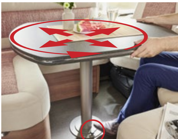
Living area table: can be conveniently rotated and moved using a foot pedal
