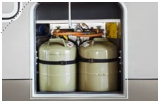
Extra-low "easy change" gas bottle compartment, one-handed hatch operation, convenient replacement of individually accessible gas bottles
