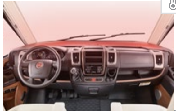
Additional heating of the driver's cabin area from the heated dashboard surface, therefore less cold radiation into the driver's cabin / living area through the windscreen
