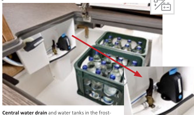
Central water drain and water tanks in the frost- proof double floor; can also be operated from the outside through the main cabin door
