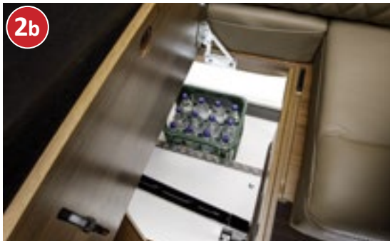
Easy removal of storage compartment contents from the inside via the swing-up seat bench cover of the L-shaped lounge seating group
