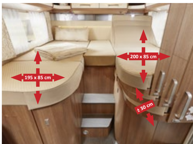
Registered for patent: Single bed can be moved by 30 cm for comfortable living and sleeping conditions within a short vehicle length (I 144 LE)
