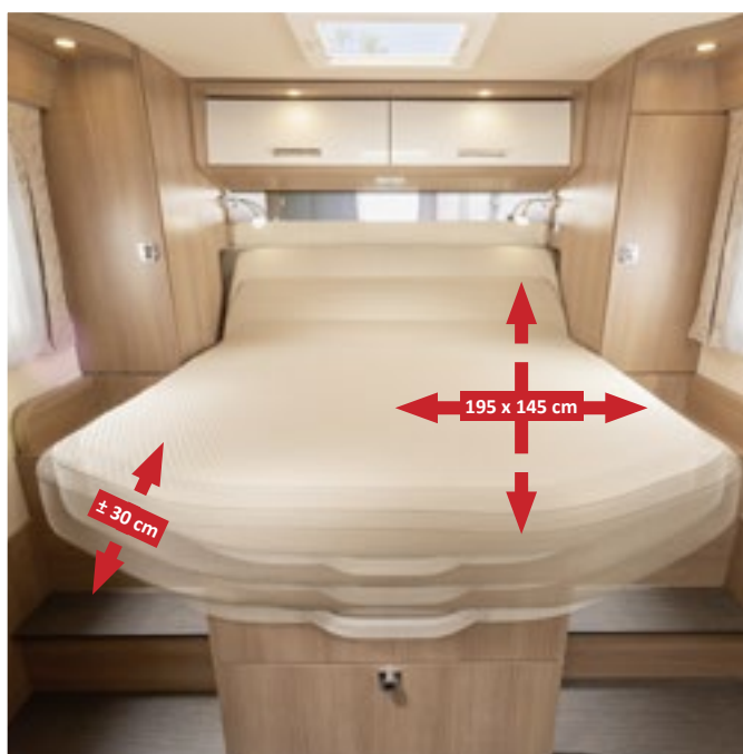
Registered for patent: Sleeping area can be moved by 30 cm for comfortable living and sleeping conditions within a short vehicle length (I 144 QB)
