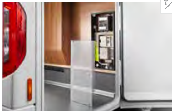
Easily accessible electrical centre in scooter garage
