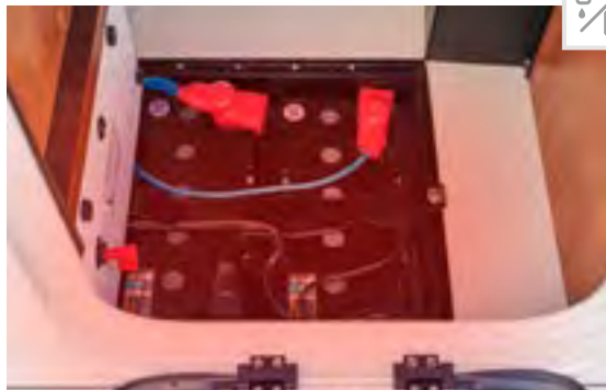
Heated battery centre with main power switch. Standard: Gel batteries 2 x 80 Ah, easily accessible, optional Lithium ion battery, 90 Ah including battery computer and separate touch display.
