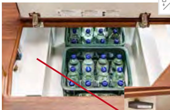
Central water drain and water tanks in the frost-proof double floor; can also be operated from the outside through the main cabin door
