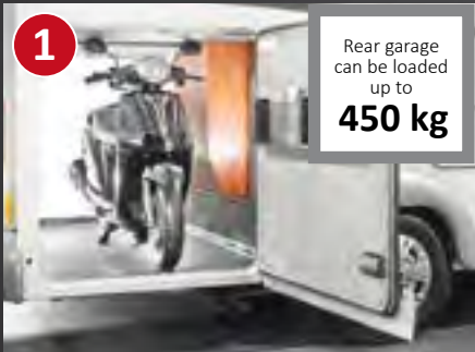
Scooter garage with considerable interior height thanks to deep lowering, accessible at both sides via a large door at the passenger side and a second door at the driver's side
